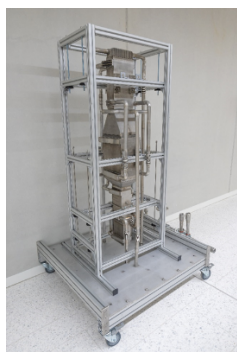
Figure 2. Microstructured ammonia decomposition processor for 21 kg/h ammonia feed
